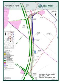
The Harwell Link Road will consist of 1.2k of single carriageway with a roundabout tying into the A417 & the A4493 with footpath, cycleway & bridleway connecting to the existing Driftway Bridleway.
